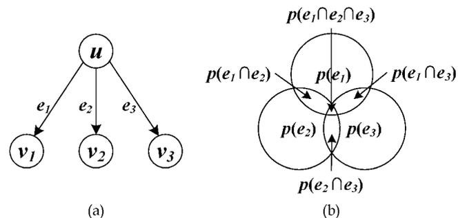
Fig. 2. Three covered nodes case. (a) A forwarder with 3 covered nodes. (b) Joint reception.
