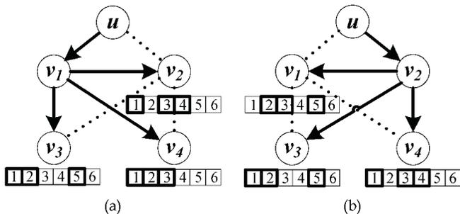
Fig. 1. Impact of coding opportunity on broadcast. In the packet reception bitmap, a block with a thick borderline means received packets, a block with a thin borderline means a lost one. (a) Case 1:  $v_1$  is the forwarder. (b) Case 2:  $v_2$  is the forwarder.
