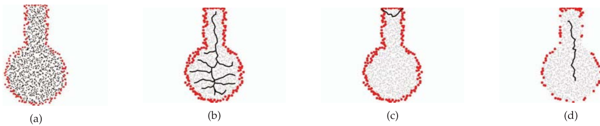
Fig. 3. Skeleton of a bat-shaped network with 1,272 nodes, average degree 13.30. (a) Original network. (b) Skeleton extracted by MAP. (c) Skeleton extracted by CASE. (d) Skeleton extracted by DIST using only 40 percent of the boundary nodes.
