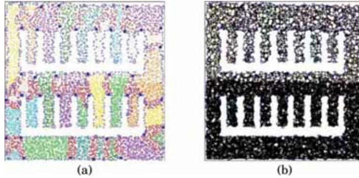
Fig. 13. Impact of non-uniform node distribution, where the upper half of the topology has node density as half as that of the lower half. (a) Topology and partitioning result. (b) Topology with links.
