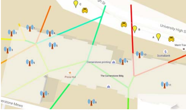
Fig. 10: An experiment scenario. The noisy reading by GPS is mapped to the true location of bus on a one-way road segment. The WiFi APs are numbered and the lines represent the Voronoi edges of SVD generated by the APs. The locations A, B, C are ground truth of the bus position by GPS, and the estimated locations are marked by the yellow bus shapes.
