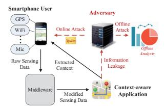
Fig. 2. A mobile phone context sensing system.
