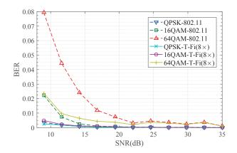
Fig. 9. BER for different modulations.
