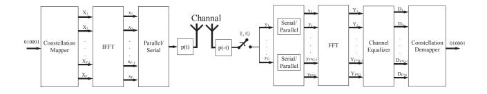
Fig. 2. OFDM schematic under overclocking.
