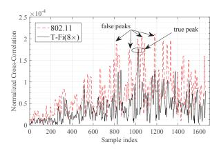
Fig. 4. Cross correlation responses at various clock rates. We set up a USRP link to capture raw data samples pf a real Wi-Fi packet at  $8\times$  and  $1\times$  Nyquist rates, respectively.
