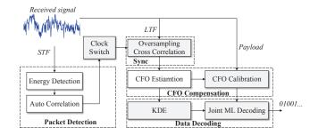
Fig. 6. System architecture of T-Fi.
