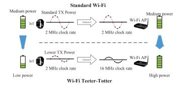
Fig. 1. The concept of Wi-Fi Teeter-Tooter. A IoT device lowers its TX power and pushes all decoding and energy burdens to the AP side. As the compensation for decreased TX power, the AP takes full advantage of its high clock rate.
