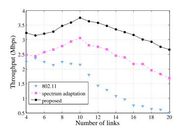
Fig. 4. Throughput under various numbers of links.
