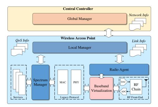
Fig. 2. SDWN-enabled system architecture for spectrum management.
