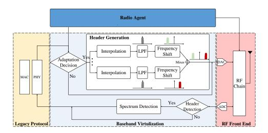
Fig. 3. Architecture of baseband virtualization.
