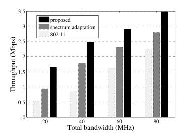
Fig. 5. Throughput under various total bandwidths.
