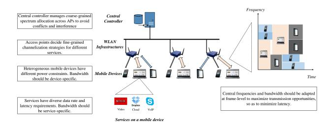
Fig. 1. Illustration of fine-grained spectrum management.
